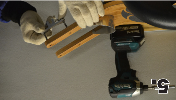
5. Place back the aluminum parts to their original position on the bottom of the fork.
