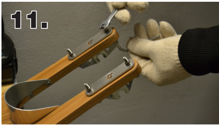
11. Lock the nuts tight using the 8mm wrench and the 4mm hex key. Always tighten with the wrench instead of the hex key for the best result.
