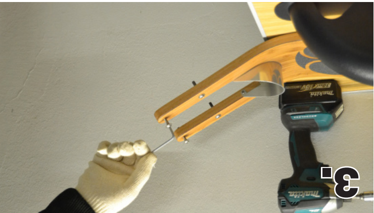
3. Remove the screws holding the aluminum part. Use the 3mm hex key for this step.
