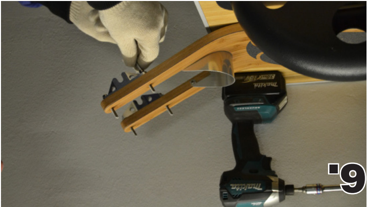
4. Prepare the two aluminum parts as shown by using all four M5X40 type screws and put 2 (i) pieces of the smaller screw washers on each screw.
