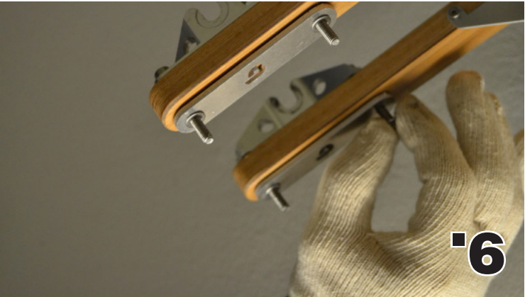
9. Place one smaller screw washer onto each screw.
