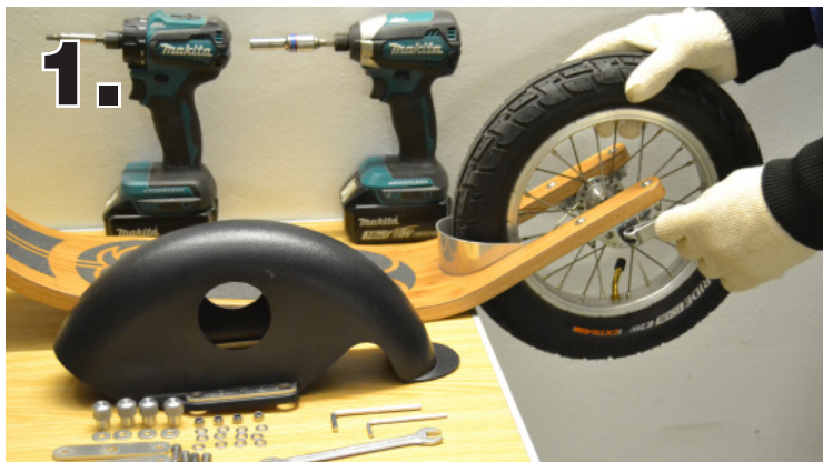
1. Loosen the rear wheel Quick Release and remove the rear wheel.
