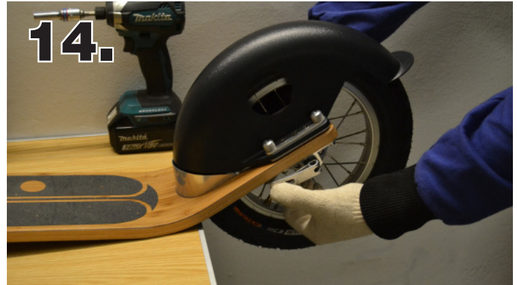
14. Put back the rear wheel into its position and secure the Quick Release.
