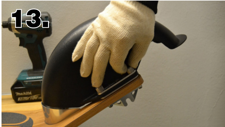
13. Lock the mudguard tight using the four thumb screw nuts.
