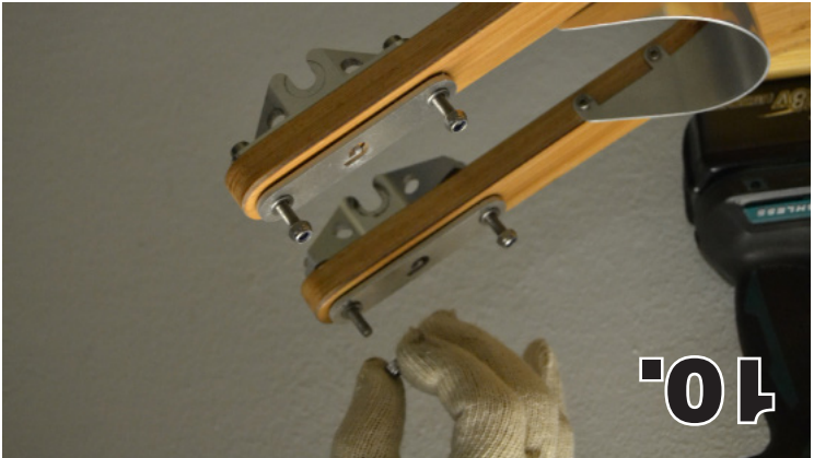
10. Place one M5 safety nut on each of the screws.
