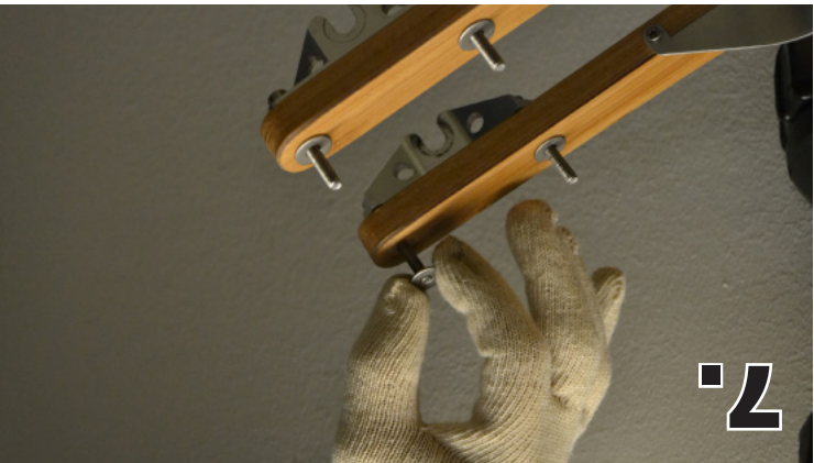
7. Place one larger screw washer onto each screw.
