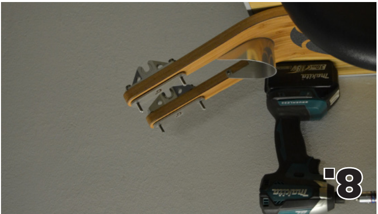
8. Place the supplied aluminum plates as shown. Mind the direction of the logo.
